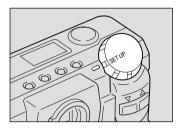
Press the button to select or [FORMAT] and press the ENTER button.
